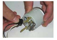
STEP 3: Insert the gauges into the housing in the locations shown.
