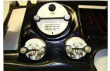
NOTE 2: This picture shows connection of lighting as would appear on Series II gauges. A separate blade terminal for power and ground exists for the internal lighting. The speedometer and tachometer have a specific lamp terminal within the 8 cavity plug.
